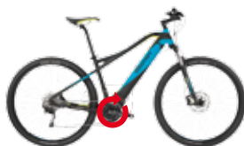
Central Motor System
